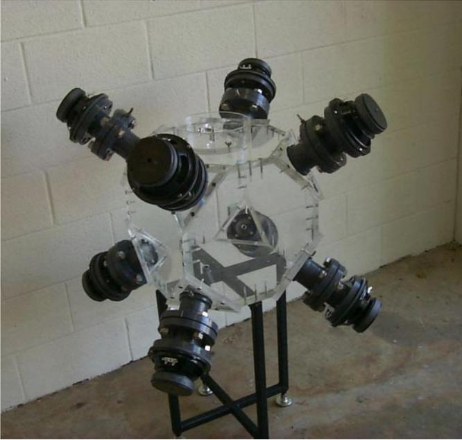
**Fig. 2.** Photograph of the turbulence chamber and actuators
