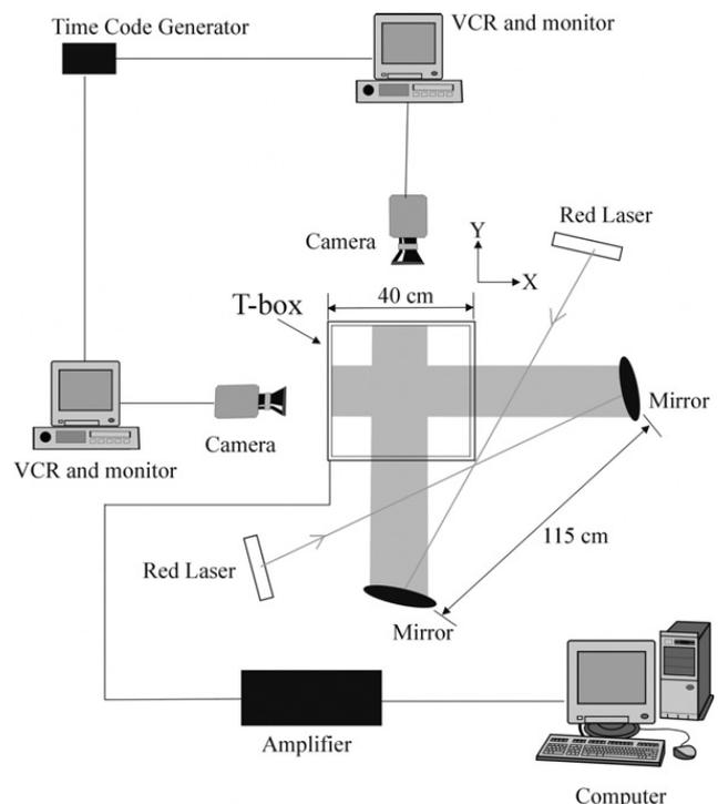
Fig. 1. Schematic of the experimental set-up during animal behavior measurements (top view).
