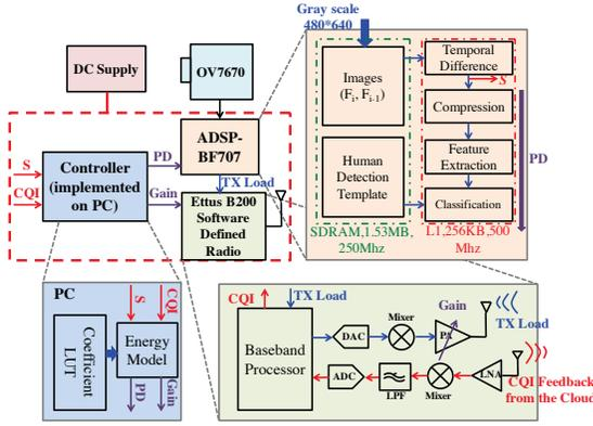
Figure 2: System architecture showing the different hardware components, the image processing pipeline (IIP) and the software defined transceiver. CQI is the channel quality index quantified by path-loss and  $S$  is the information content size defined in the following section.
