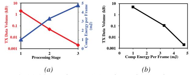
Figure 4: (a) Measured transmission data volume and computation energy vs processing depth. (b) Estimated transmission data volume vs. computation energy.
