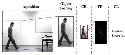
Figure 3: Algorithm demonstration with a real video frame. The system first locates and segments moving object from captured raw image and further compresses the segmented sub-image; then the feature descriptor will be extracted from the compressed object in feature extraction stage (FE) and fed to the template in the last stage for final classification (CL).
