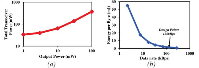
Figure 5: Measured (a) transceiver power vs. output power. (b) energy per byte vs. data rate.
