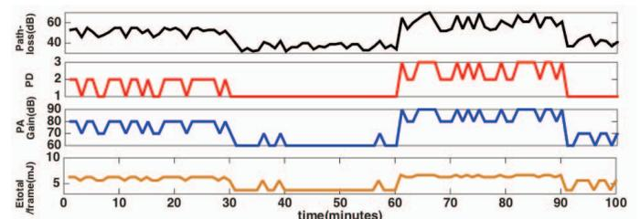
Figure 10: Case study for mobile sensor node with varying path-loss and correspondingly self-optimizing PD, PA gain, and total energy/frame.
