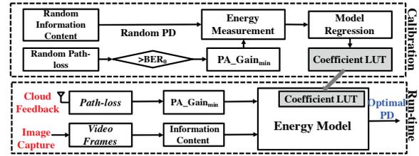
Figure 8: Flow-chart illustrating test/calibration and run-time self-optimizing.
