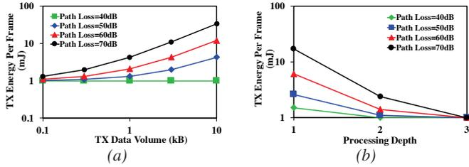
Figure 7: Measured (a) transmission energy per frame vs transmission data volume under various channel conditions. (b) Transmission energy per frame vs. processing depth under different path-loss conditions.
