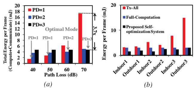
Figure 9: (a) Measured total energy per frame under different path-loss conditions and processing depth. The optimal processing depth is denoted in the figure. (b) Average energy consumption per frame under various environments using different strategies.
