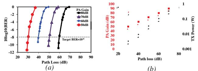
Figure 6: Measured (a) bit-error-rate vs. channel path loss with different PA gain. (b) PA gain and transceiver power vs. path loss for adaptive radio at target BER of 10<sup>-8</sup>.
