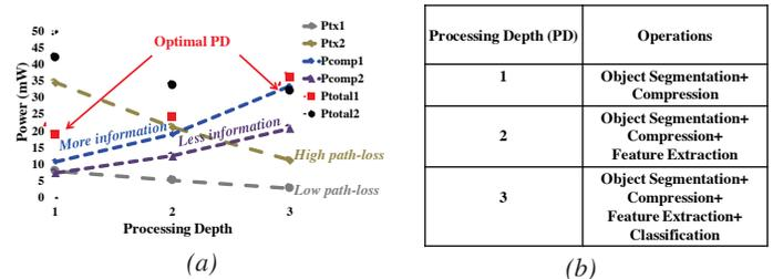
Figure 1: (a) Power consumption changes with PD and the optimal PD for minimum-power consumption also varies under different channel conditions and information content: noisy channel and small information, thus light computation, result in more embedded processing and vice versa. (b) Operations included in each processing depth (PD).
