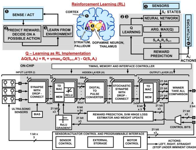
Figure 7.4.1: Motivation and system diagram for reinforcement learning as a neuromorphic computational model in autonomous mobile micro-robots.
