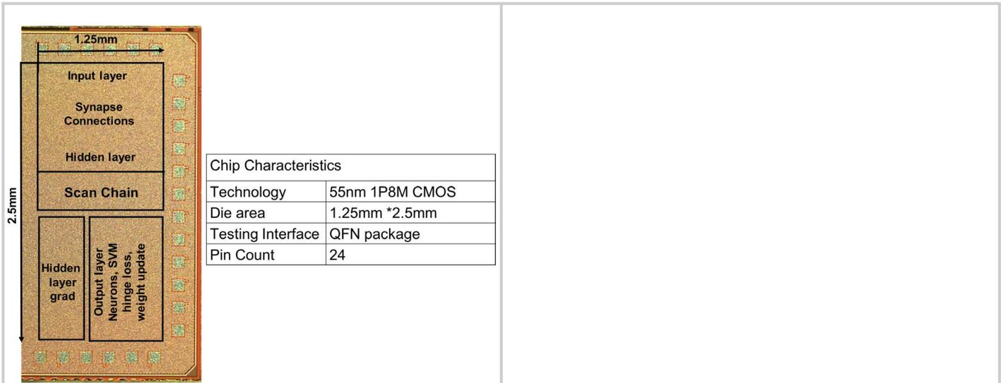
Figure 7.4.7: Die-photo and chip characteristics.
