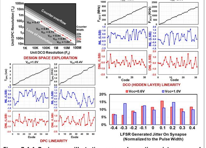
Figure 7.4.4: Design space illustrating measured operating points, measured DCO characteristics, measured DPC characteristics and measured stochasticity generated by the synapses.
