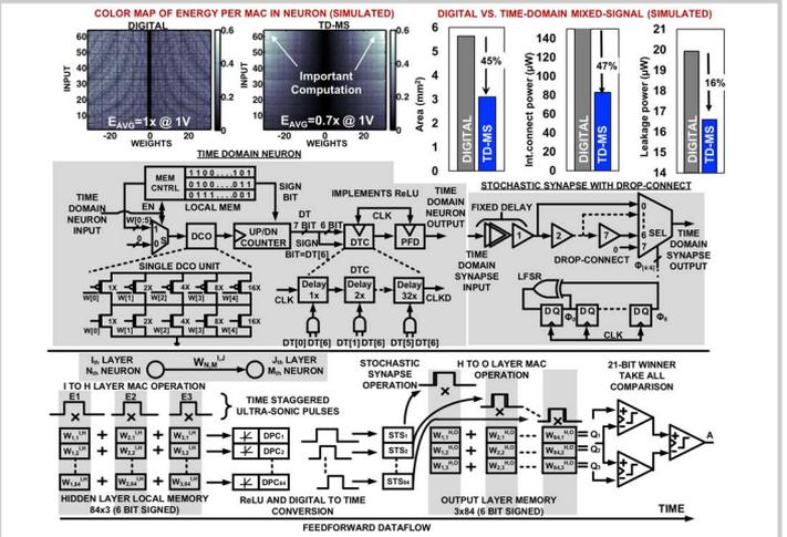
Figure 7.4.2: Comparison of time-domain mixed-signal (TD-MS) design vs. digital implementation, design of TD-MS neuron with ReLU, stochastic synapses and feedforward timing diagram illustrating pipelined data-propagation.
