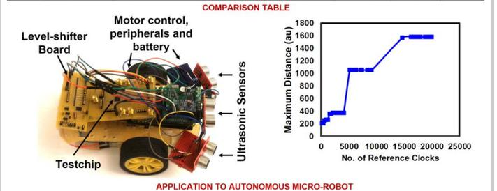
Figure 7.4.6: Comparison table and application to mobile micro-robotics illustrating the use of RL in exploration.
