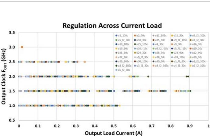
Figure 19.3.5: Measured UVFBR output clock frequency ( $F_{OUT}$ ) regulation vs. output load current for temperature ranging from  $-15^{\circ}\text{C}$  to  $105^{\circ}\text{C}$  across 24 dies.
