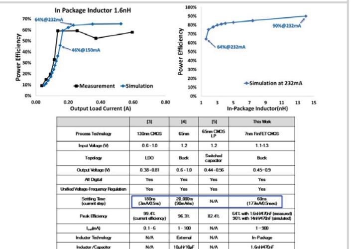
Figure 19.3.6: Measured and simulated UVFBR power efficiency vs. output load current and in-package inductor size and comparison table with other unified voltage-frequency regulation designs.
