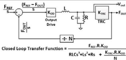
Figure 19.3.3: UVFBR small signal analysis and simulated UVFBR loop gain and phase.
