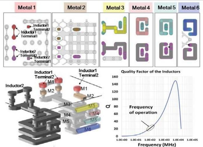
Figure 19.3.2: 3D view of the six metal levels for the two in-package inductors, a detailed view of each metal layer, and the simulated inductor quality (Q) factor. Q ranges from 17 to 30 in the region of operation.
