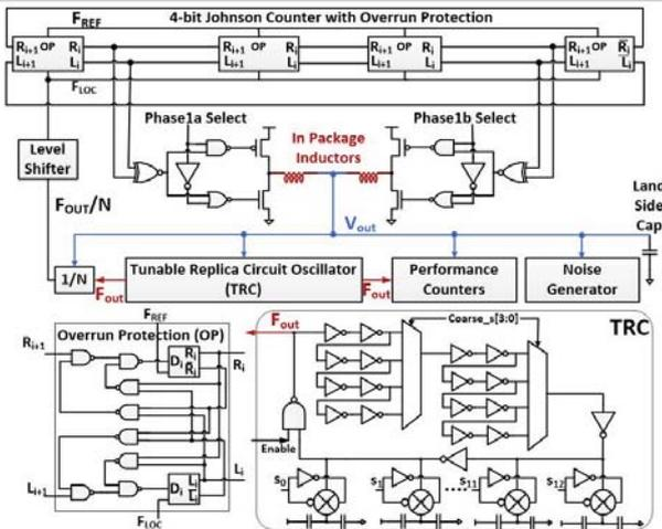
Figure 19.3.1: Test-chip block diagram of the UVFBR with two in-package inductors, performance counters, programmable noise generators, and schematics of the 4b Johnson Counter with overrun protection, and the tunable-replica circuit (TRC) oscillator.
