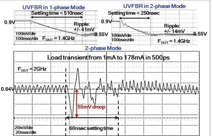
Figure 19.3.4: Measured oscilloscope captures the UVFBR 1-phase and 2-phase modes during a 0.9V to 0.55V ( $F_{OUT}=1.4\text{GHz}$ ) transition and the UVFBR transient response ( $F_{OUT}=2\text{GHz}$ ) in 2-phase with a current load step from 1mA to 178mA at a rise time of 500ps.
