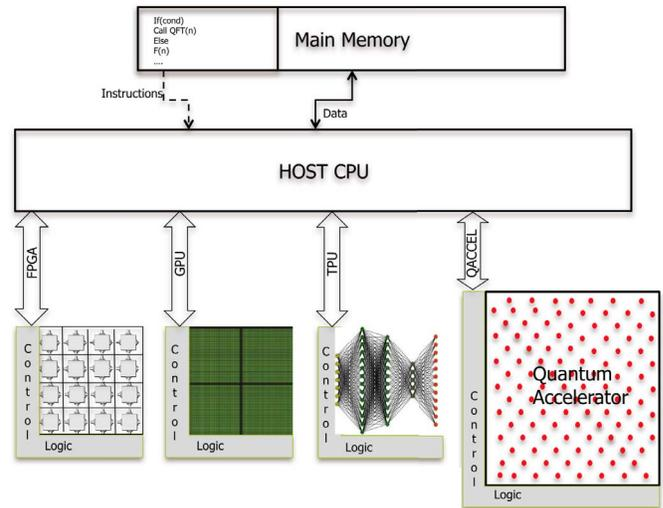
Fig. 1: System architecture with heterogeneous accelerators.
