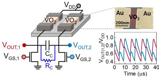
**Fig. 3:** An IMT device coupled through its Resistive and Capacitive elements showing frequency locking.
