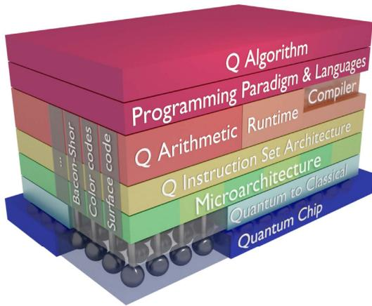
**Fig. 2:** The required layers of a Quantum Computer.
