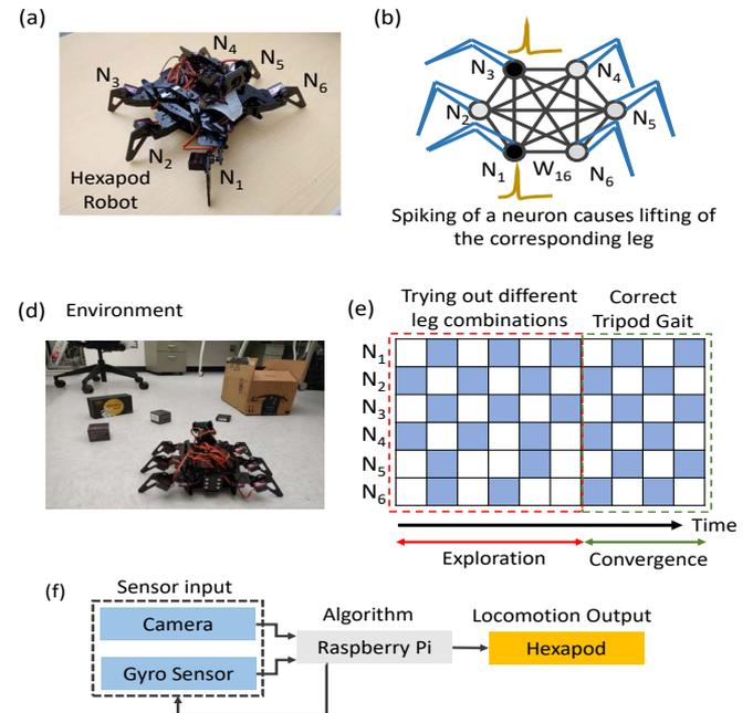
Fig. 1. (a,b) Hexapod robot with labeled neurons for mimicking the CPG. Spiking of a neuron causes motion of the corresponding leg (c) Office environment for demonstration (d) SCPG spiking as the algorithm progresses. The random spiking in the exploration phase gets latched to the correct tripod gait showing convergence (f) Hardware implementation of the system
