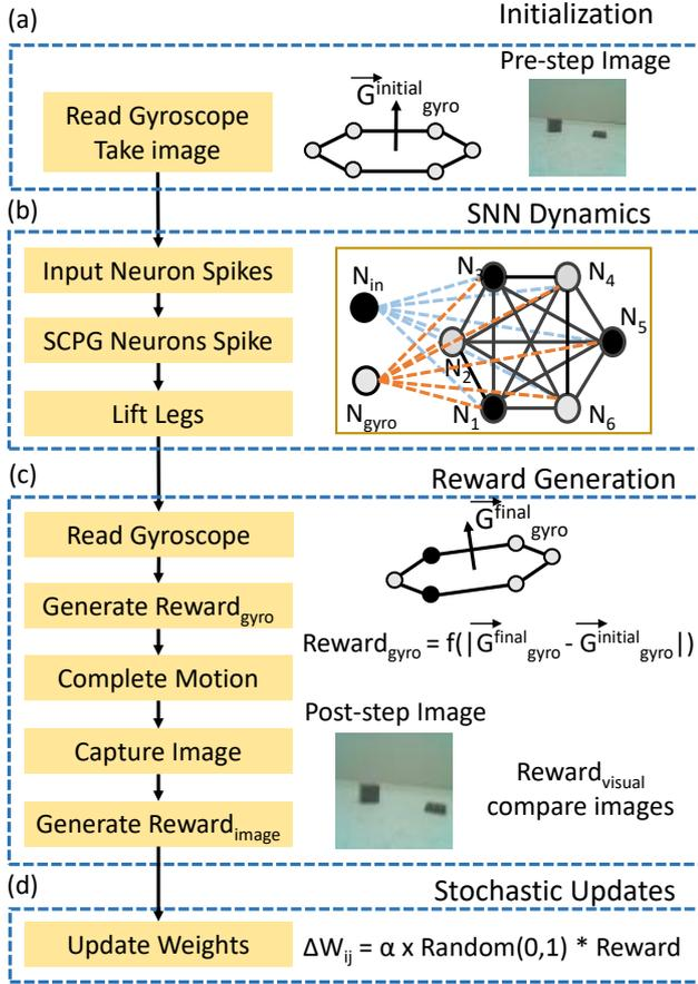
Fig. 2. Block diagram of the algorithm (a) Every step is initialized with a gyroscope reading and an image of the surroundings (b) LIF neuronal dynamics compute the spiking of the neurons (c) Sensory inputs are used to calculate the awards (e) Weight update using calculated rewards
