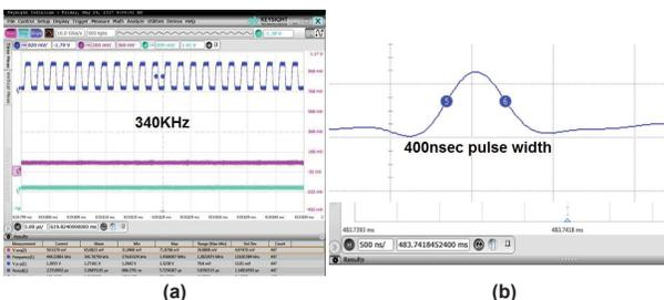
Fig. 12: (a) Scope capture of the VCO frequency at 360mV (b) Zoomed-in scope-capture of the DPC output
