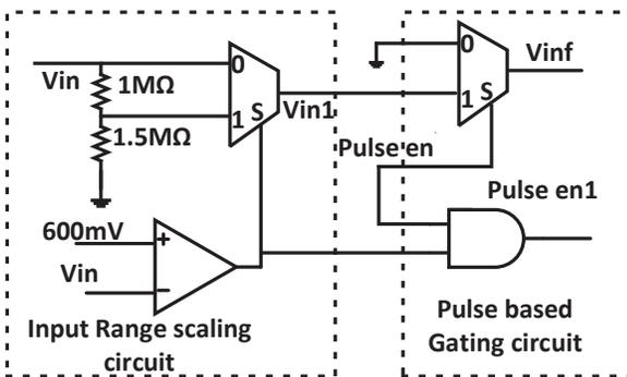
Fig. 5: Input dependent scaling of the output code achieves input range extension
