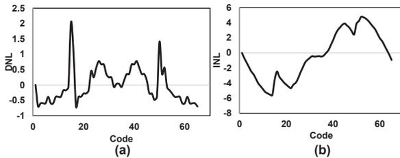
Fig. 10: (a) Measured DNL of the proposed front-end (b) Measured INL of the proposed front-end
