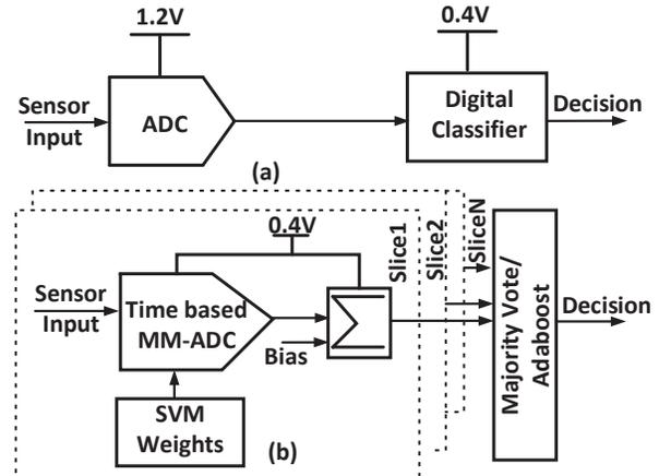
Fig. 1: (a) Traditional sensor/classifier interface (b) Proposed sensor/classifier interface
