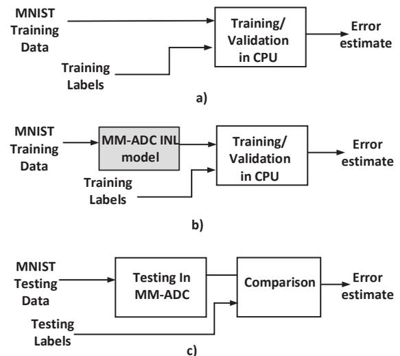
Fig. 8: (a) Traditional training procedure (b) Proposed INL aware training and (c) Testing for accuracy of inference
