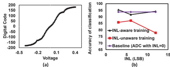
Fig. 11: (a) Digital code vs differential input voltage (b) Classification accuracy for a baseline design and TD ADC based design with and without error aware training
