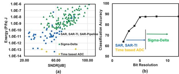
Fig. 2: Choice of ADC for in-situ matrix multiplication
