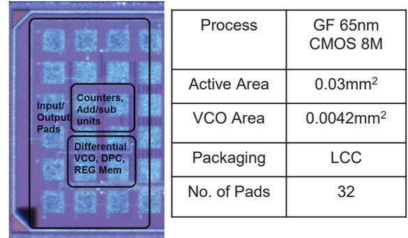
Fig. 7: Die shot and chip characteristics
