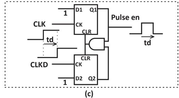
Fig. 6: Digital to pulse converter (DPC) for pulse generation
