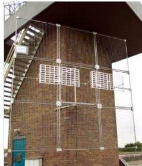
Figure 9: NATO NC3A antennas: a.) transmitter (left), b.) receiver (right).
