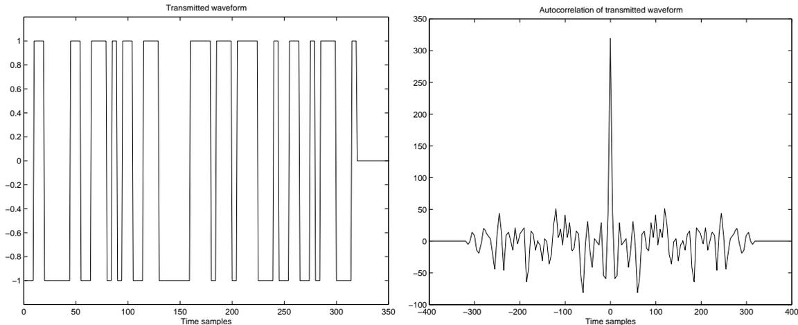
**Figure 2.** Left panel: Transmitted waveform. Right panel: Autocorrelation of transmitted waveform.
