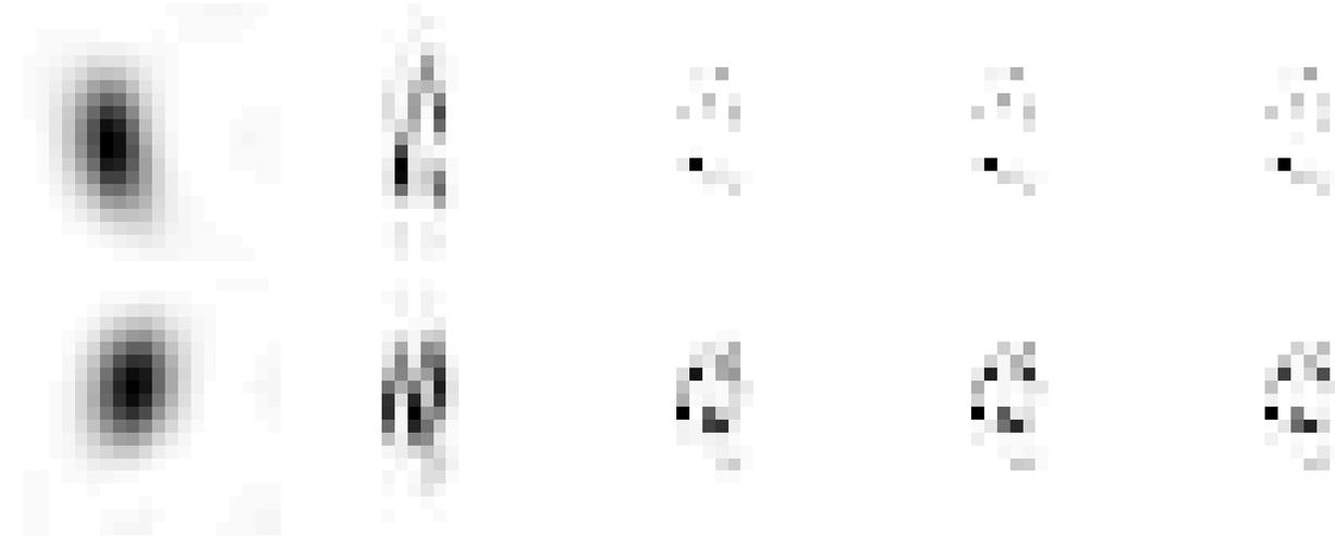
**Figure 8.** Matched-filter output and EM iterations for specular data generated from the sphere. Leftmost column shows the squared magnitude of the matched-filtered output. From left to right, the remaining columns show results at 1, 5, 10, and 20 iterations. Top and bottom rows correspond to different specular data realizations.
