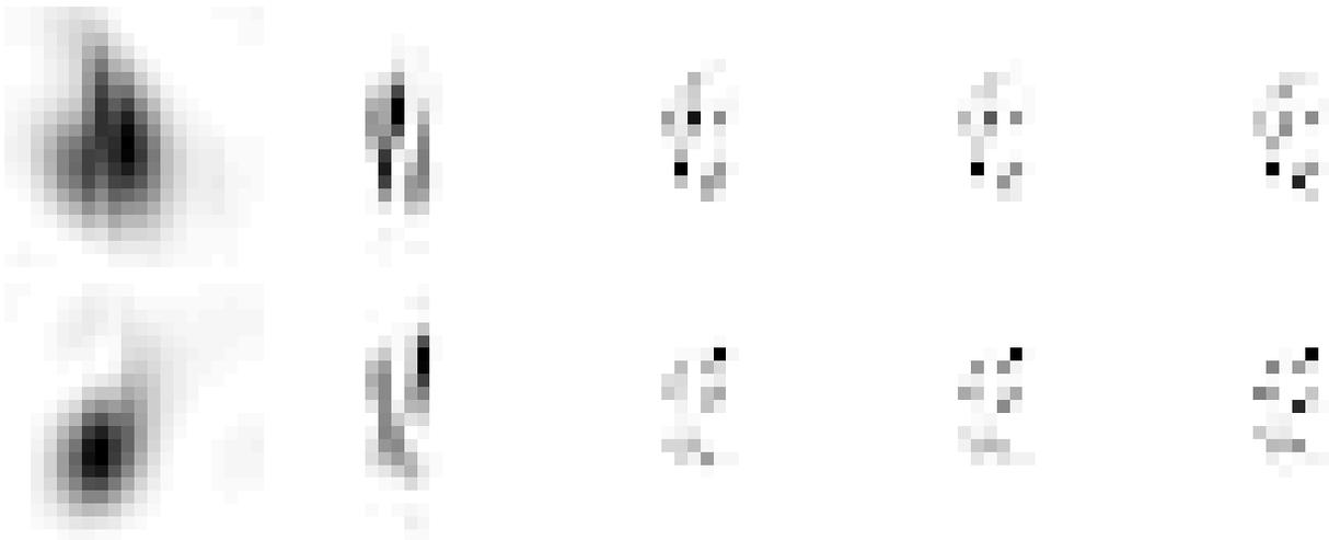
**Figure 7.** Matched-filtered output and EM iterations for diffuse data generated from the sphere. Leftmost column shows the squared magnitude of the matched-filtered output. From left to right, the remaining columns show results at 1, 5, 10, and 20 iterations. Top and bottom rows correspond to different diffuse data realizations.
