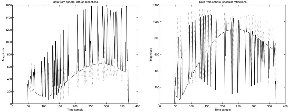
**Figure 6.** Magnitude of data from two diffuse (left panel) and two specular (right panel) realizations from the sphere. For the left panel, the solid line corresponds to the left panel of Fig. 5; dotted line corresponds to the right panel.
