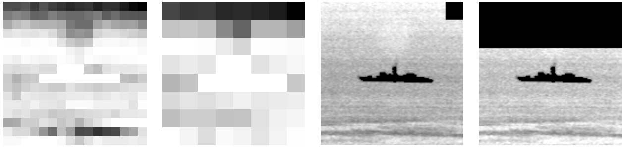
Figure 8: Additional detection following the estimation of the shape of the ship. The algorithm finds the sky, which is of greater intensity than the rest of the background.
