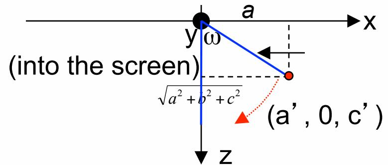
$$T_3 = \begin{bmatrix} \cos \omega & 0 & -\sin \omega & 0 \\ 0 & 1 & 0 & 0 \\ \sin \omega & 0 & \cos \omega & 0 \\ 0 & 0 & 0 & 1 \end{bmatrix}$$
