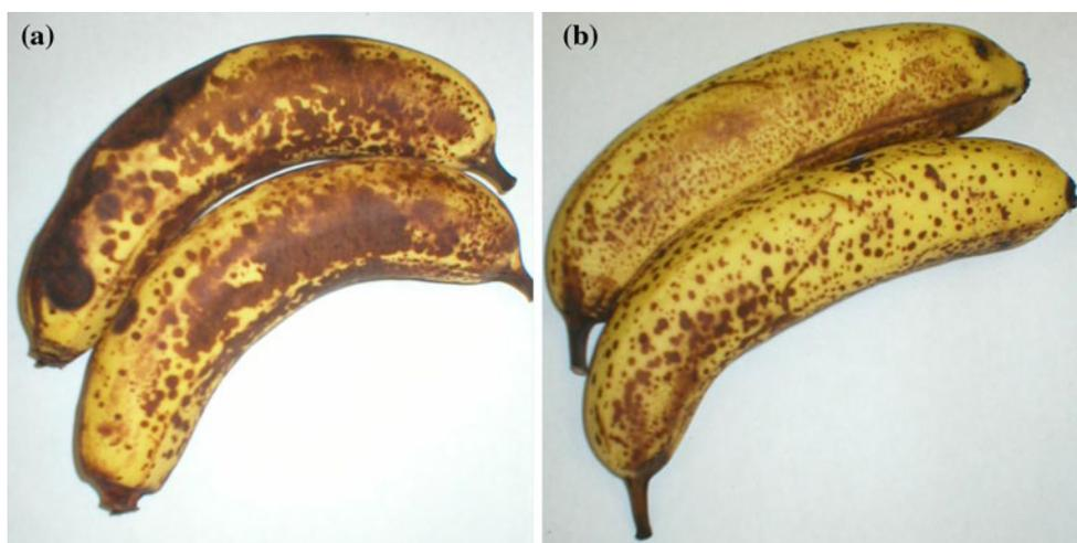
**Fig. 3** Images showing comparison of control, non-treated bananas **(a)** with bananas placed in proximity to immobilized catalyst (5 cm) **(b)** both after 7 days at ambient temperature and with humidity control
