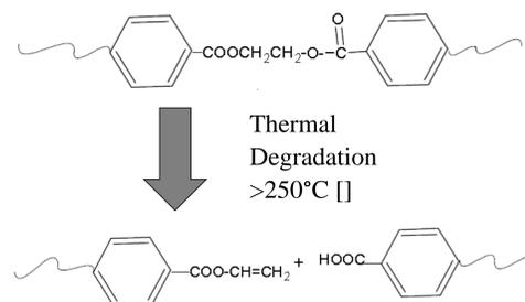
Figure 5: Traditionally challenges in recycling PET are due to its thermal degradation
