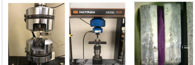
Tensile Testing Flexural Testing Tested Sample
