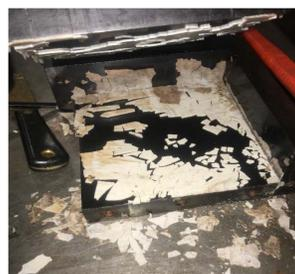
Figure 4: Compression molding; 2 hour heating time; 257°C; 1 MPa; Obvious thermal degradation
