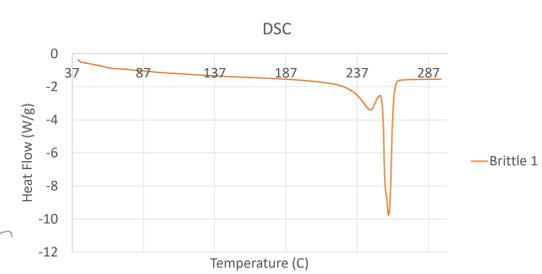
Figure 6: DSC Verification of thermal degradation
