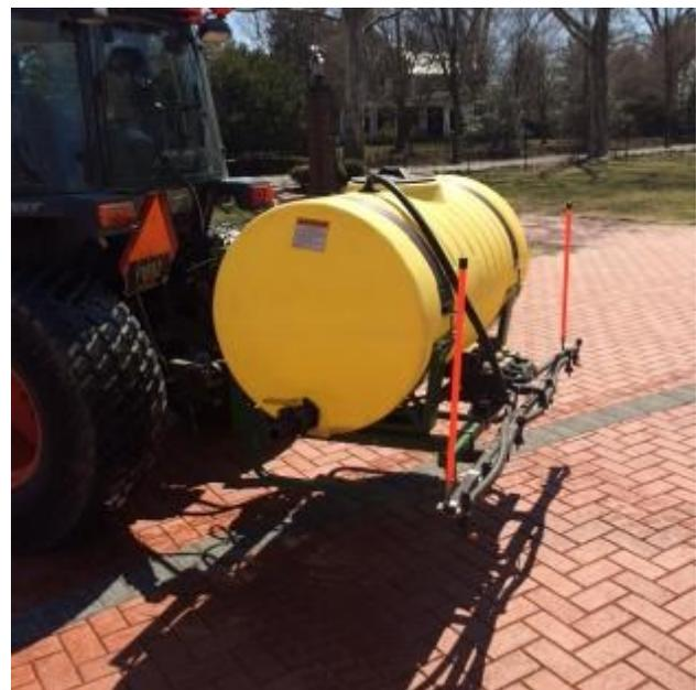
ice control program at UD. Roger Bowman, Manager of Grounds Services, observed that the anti-icing setup will, “allow us to apply brine at a controlled rate to a wide range
