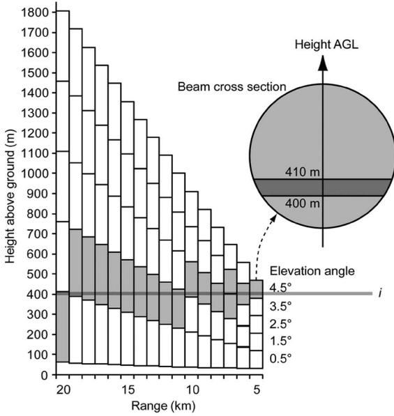
Fig. 2. Example principle of calculation of VPR. Pulse volumes within  $D_i$ , where  $i = 41$ , are shaded in gray. The radar beam cross section depicts  $\beta$ , i.e., the proportion of the beam within height interval  $i$ , for the pulse volume at  $4.5^\circ$  elevation and 5-km range.
