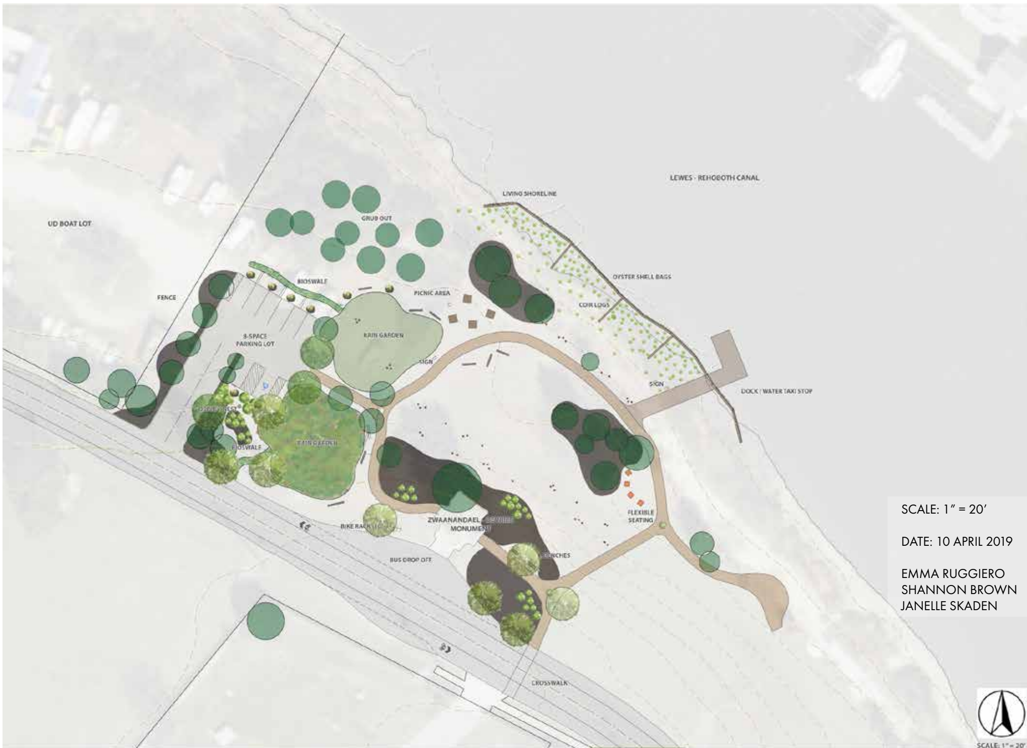
Figure 26: The mid-term design included an 8-space parking area, a dock, and a living shoreline treatment comprised of coir logs and oyster shell bags.
