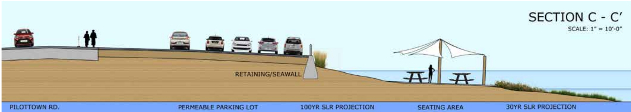
Figure 33: Section C-C' shows the parking and seating areas. The parking area will require a regrade so that all pavement is at a high elevation above the floodplain. An engineered retaining wall that allows for this regrade may function as a future seawall. The seating area features moveable shade sails clipped to tall pilings and picnic benches equipped with anchors to secure them to the pavers below. The design of this adaptable seating area allows for short term flooding without concern for floating projectiles. In the long term, all seating area elements may be easily removed except for secured pilings that may take on another use, such as a base for a floating dock.
