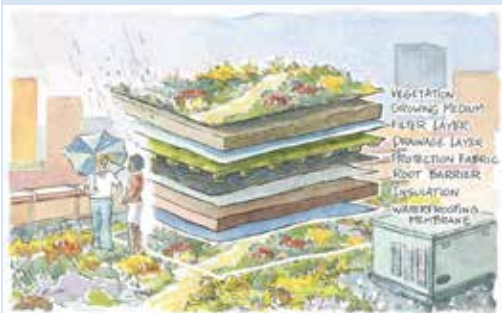
Image: Illustration of green roof layers, via Jeffery Mathison/ DNREC.
