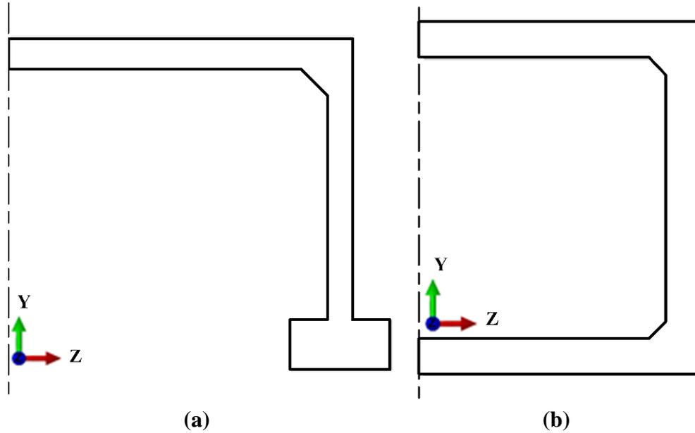
Figure 2 Typical 2-D culvert cross-section: (a) BR-1 and BR-2; (b) BR-3 and BR-4.
