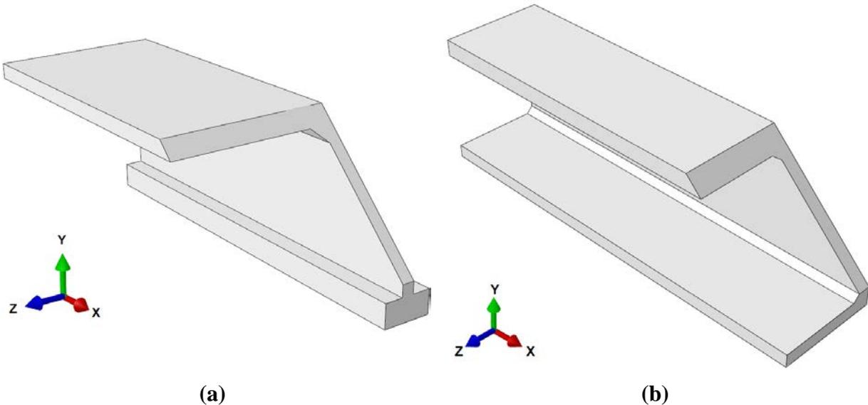
Figure 3 Typical 3-D culvert cross-section: (a) BR-1 and BR-2; (b) BR-3 and BR-4.
