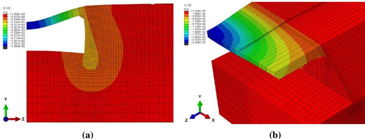
**Figure 8 Static response in BR-1 and BR-2 at maximum displacement conditions: (a) 2-D model (magnified 100 times); (b) 3-D model (magnified 300 times).**
