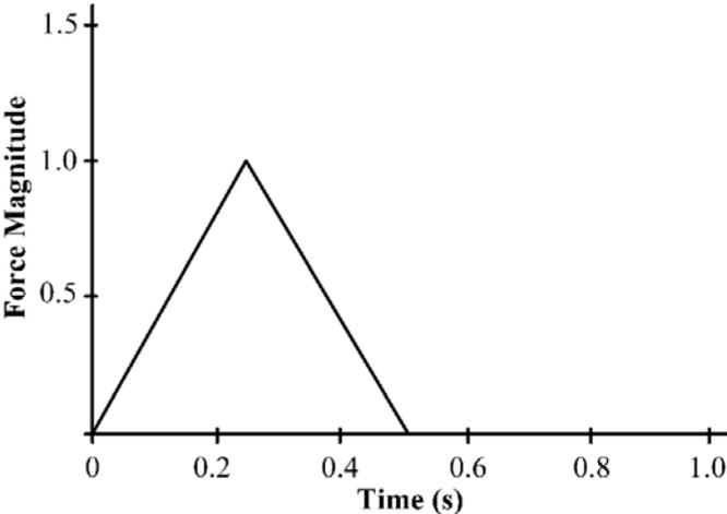
**Figure 6 Symmetric triangular pulse load.**
