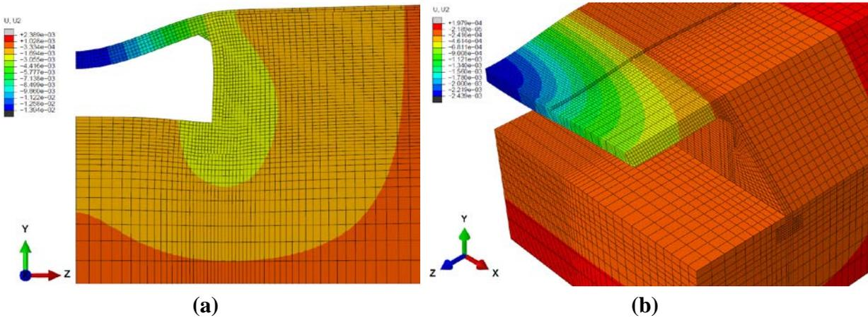
**Figure 7 Dynamic response in BR-1 and BR-2 at maximum displacement conditions: (a) 2-D model (magnified 100 times); (b) 3-D model (magnified 300 times).**
