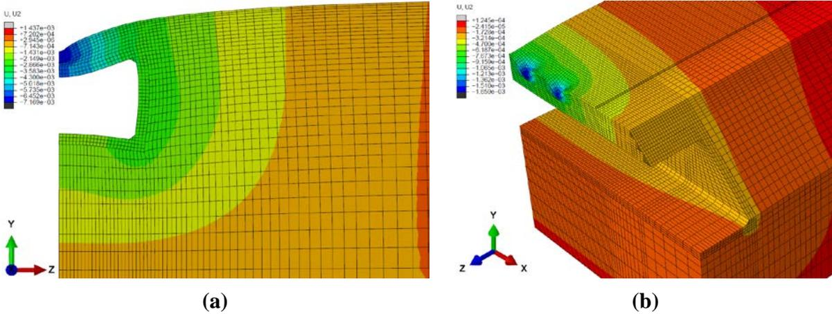
Figure 9 Dynamic response in BR-3 and BR-4 at maximum displacement conditions: (a) 2-D model (magnified 200 times); (b) 3-D model (magnified 500 times).
