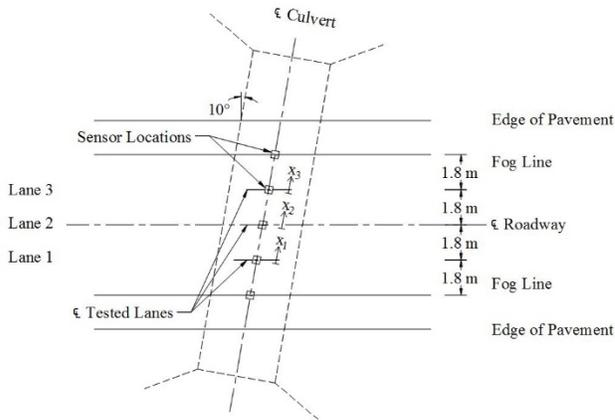
**Fig. 3** Culvert 1 Sensor Locations
