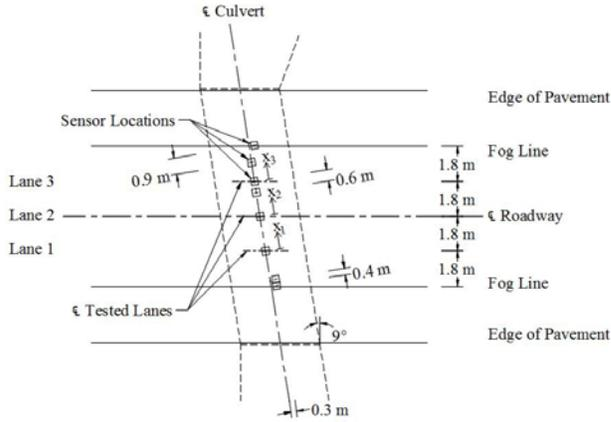
**Fig. 6** Culvert 4 Sensor Locations
