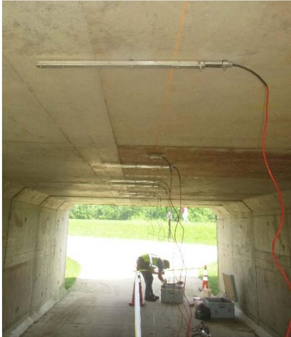
**Fig. 2** Typical instrumented culvert
