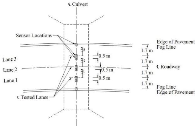
**Fig. 4** Culvert 2 Sensor Locations
