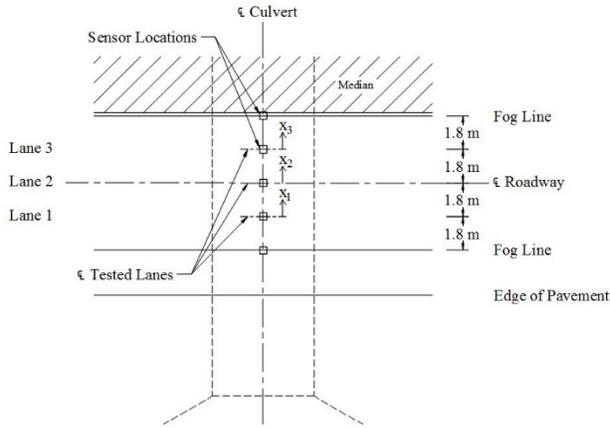
**Fig. 5** Culvert 3 Sensor Locations
