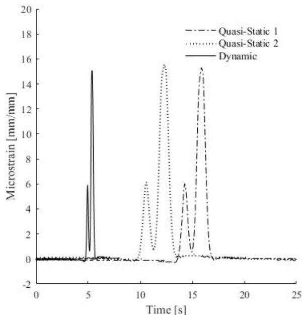
**Fig. 8** Time History Analysis of Strain in Lane 2 of Culvert 2 due to Truck 1
