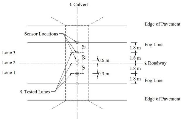
**Fig. 7** Culvert 5 Sensor Locations
