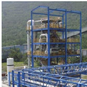
Figure 4. Multi-Functional Reactor – Chemical Looping for Carbon Dioxide Separation. Courtesy of Prof. L. S. Fan.
