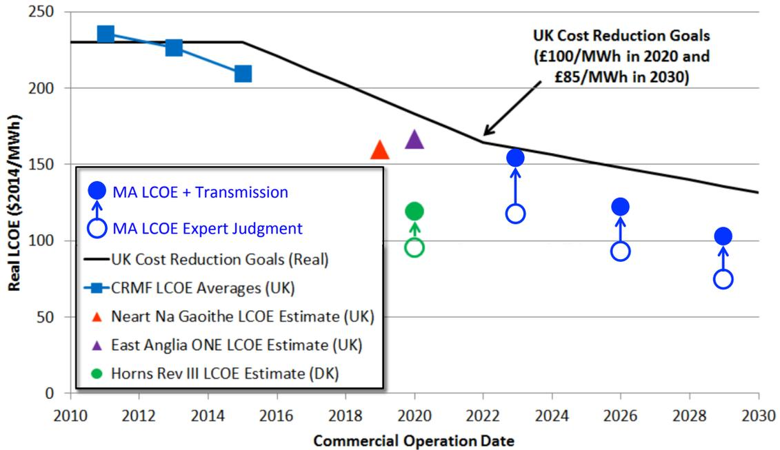
**Figure 4.** This report’s estimated Massachusetts LCOEs (blue circles) benchmarked against European LCOEs. (Original figure from NREL report, referenced in this report’s prior Figure 1.)<sup>63</sup>
