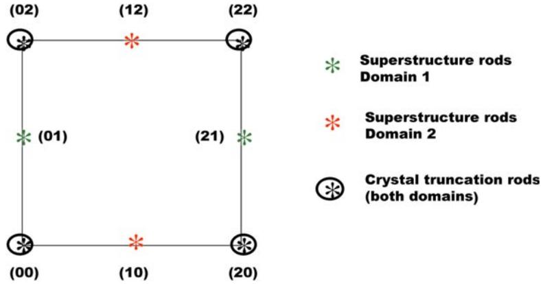
**Figure 4.** A cut through reciprocal space parallel to the surface intersecting the diffraction rods from a mixture of two mutually rotated Ge(001)-(2 × 1) domains. Marked by black asterisks surrounded by circles are the CTRs with contributions from both substrate and surface scattering. The red asterisks mark the positions of the superstructure rods from the left-hand model domain of figure 3, while the green asterisks mark those from the right-hand model domain of the same figure.
