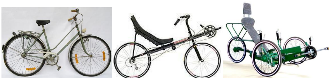
Figure 1. An upright bicycle, a recumbent bicycle, and a rigid recumbent tricycle, from left to right. (all images from Wikimedia Commons)
