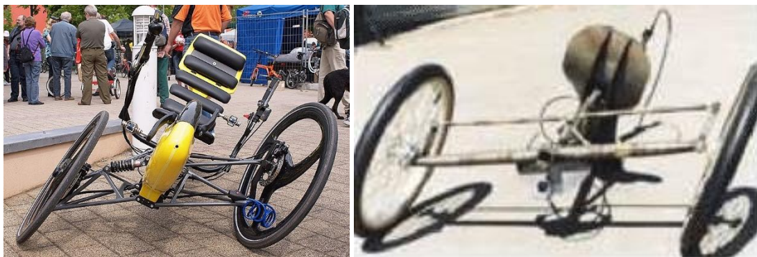
Figure 3. Tripendo and Paul Sims’ openly documented parallelogram tilting tricycle.
