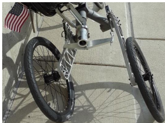
Figure 4. Bell crank, tie rod, and swing arm mechanism.
