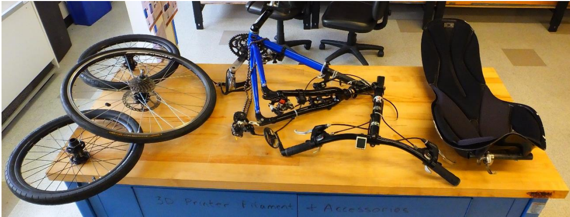
Figure 20. Cruzbike front frame, along with wheels, seat, stem, and handlebars.
