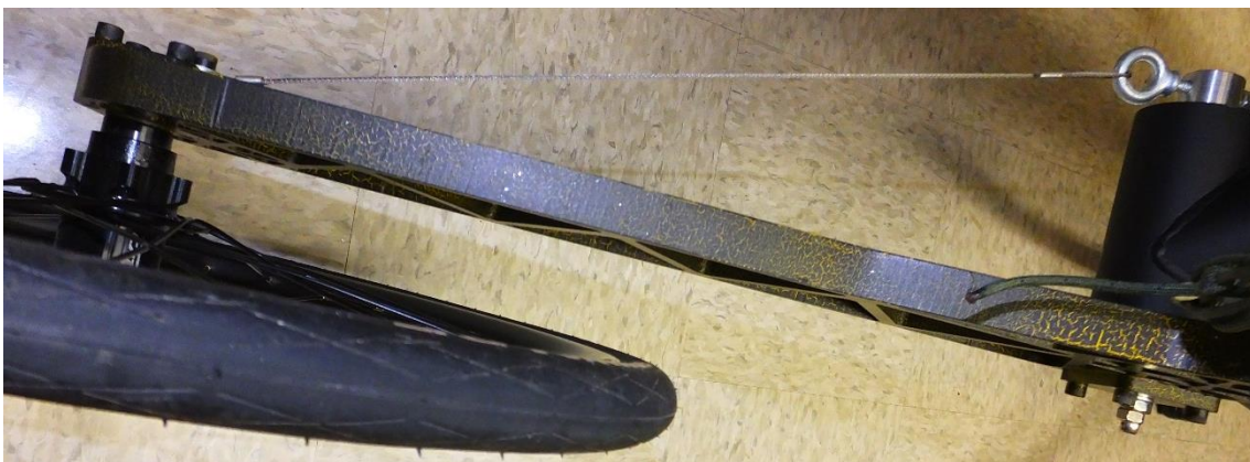
Figure 22. Damping lanyard (thin, silver-looking wire) from swing arm end to pivot axle.
