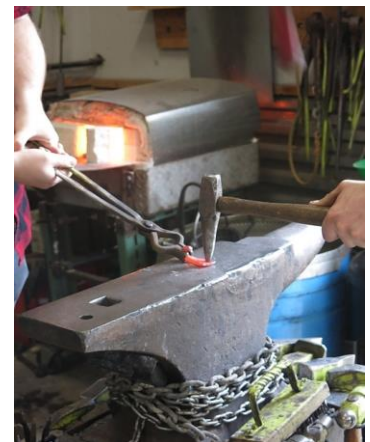
Adding rivet holes to the hook. Photo: Stanton
