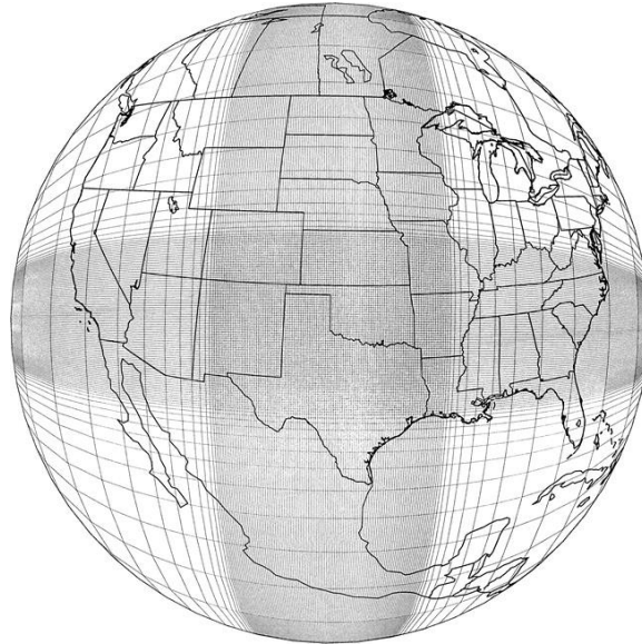
Figure 9. An example of a stretched horizontal grid. In this example, the full limited-area model domain is 353 x 415 grid points, with the centermost 240 x 323 grid points having uniform horizontal resolution. The horizontal grid spacing decreases by 10% per each model grid length as one moves from the periphery of the limited-area domain, where it is identical to that of the global model used to initialize and provide lateral boundary conditions to the simulation ( 2^\circ ), to the center of the limited-area domain, where it is 0.04^\circ . Figure obtained from Yeh et al. (2002, Mon. Wea. Rev. ), their Fig. 6.
