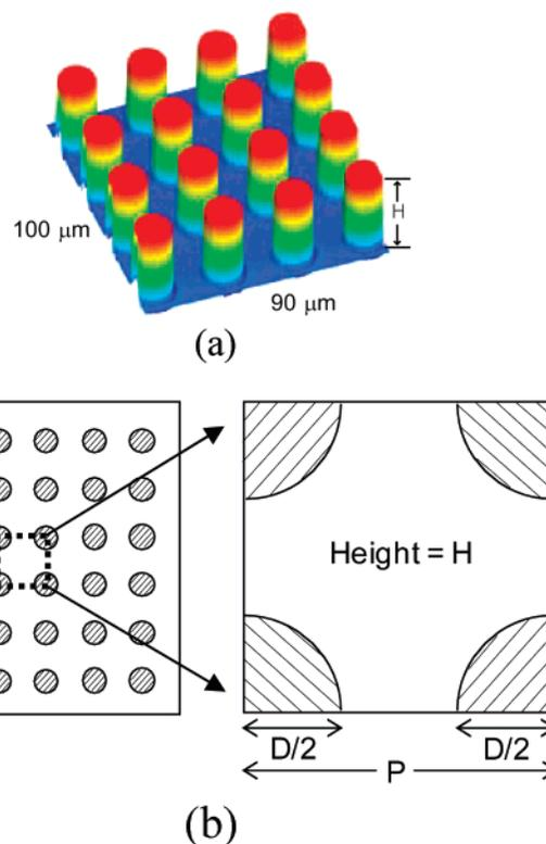
**Figure 5.** (a) Optical profiler image and (b) schematic of the patterned surface.
