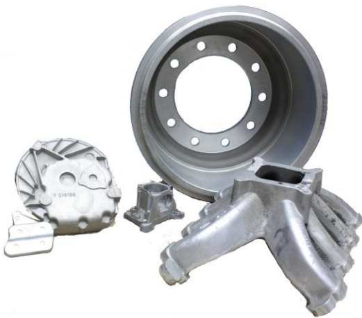
Fig. 4 — Automotive components made of aluminum- and magnesium-fly ash composites developed at UWM[12].
