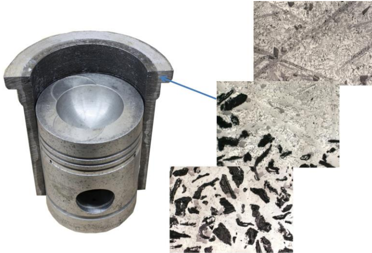
Fig. 1 — Aluminum-graphite particle composite piston and cylinder liner developed at UWM Center for Composite Materials. The inset microstructure shows that graphite particles concentrate in the inner periphery of the liner.
