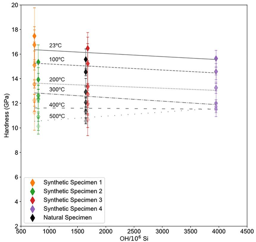
**Figure 2.** Hardness values for each specimen indented parallel to [0001] plotted against hydroxyl concentration as measured by secondary ion mass spectrometry (SIMS). Best-fit lines are drawn to connect measurements at equivalent temperatures. Lighter points represent higher temperatures.
