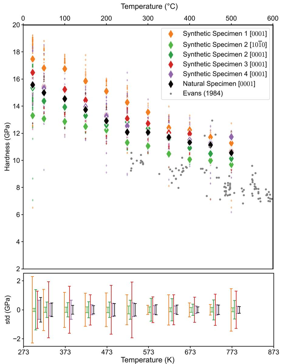
**Figure 1.** Indentation hardness decreases as a function of temperature. Small diamonds are individual measurements; large diamonds are averages at each temperature. Microindentation data from Evans (1984) is shown in gray circles. Error bars at each temperature are arbitrarily offset for clarity and represent  $\pm$  one standard deviation. Only indents for ill-behaved load functions have been removed.
