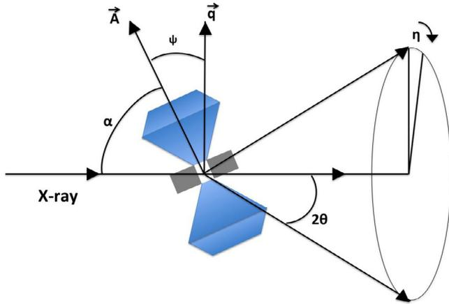
**Fig. 1.** Schematic for the setup of a radial diffraction experiment. The incident monochromatic X-ray beam is nearly perpendicular to the compression direction of a non-hydrostatically loaded DAC.  $2\theta$  is the diffraction angle;  $\eta$  is the azimuth angle;  $\psi$  is the angle between the diamond compression axis and the momentum transfer; and  $\alpha$  is the angle between the diamond compression axis and the X-ray beam.
