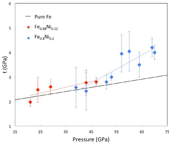
**Fig. 3.** A comparison of the strengths of pure Fe,  $\text{Fe}_{0.88}\text{Ni}_{0.12}$ , and  $\text{Fe}_{0.8}\text{Ni}_{0.2}$  at high pressure and room temperature. Trend for pure Fe was calculated from Gleason and Mao, 2013 (black line). Dotted lines are linear fits for  $\text{Fe}_{0.88}\text{Ni}_{0.12}$  (red) and  $\text{Fe}_{0.8}\text{Ni}_{0.2}$  (blue). (For interpretation of the references to colour in this figure legend, the reader is referred to the web version of this article.)
