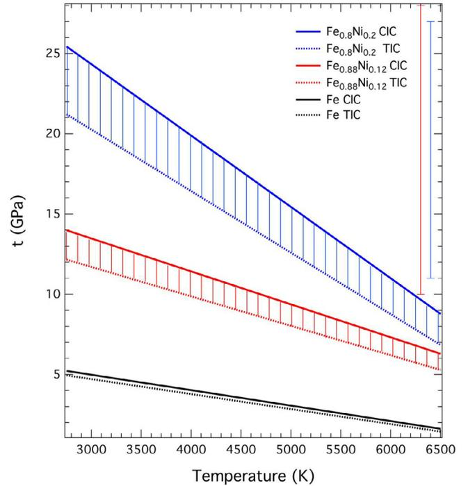
**Fig. 4.** Steinberg-Guinan temperature extrapolation (Steinberg et al., 1980) for pure Fe (Gleason and Mao, 2013),  $\text{Fe}_{0.88}\text{Ni}_{0.12}$ , and  $\text{Fe}_{0.8}\text{Ni}_{0.2}$ . Strength calculations were based on the center of the inner core (CIC); 364 GPa and 6200 K, to top of the inner core (TIC) conditions; 329 GPa and 6200 K. Representative uncertainties for both compositions at TIC pressure at 5500 K are shown at the top right.
