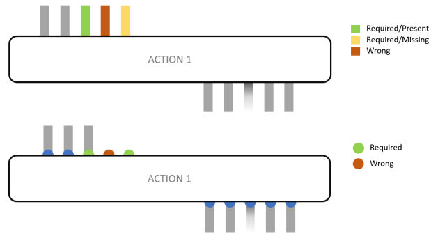
Figure 2: An action-space visualization example, with preconditions at the top of each action, and effects at the bottom. Deletion effects are represented as a flow fading out. Top: The highlight-based explanation visualization; Bottom: The port-based explanation visualization.
