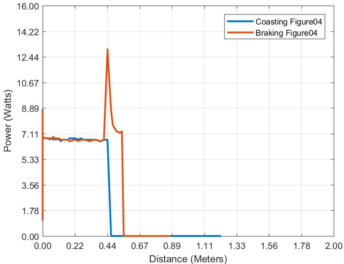
Figure 2: Power used over Distance AEV Traveled
