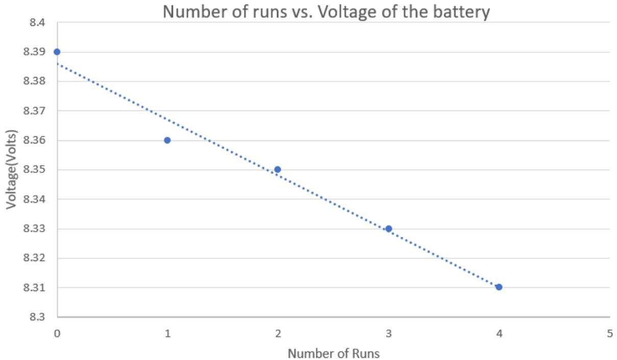
*Figure 3: Battery Voltage Relation with Number of Test Runs*
