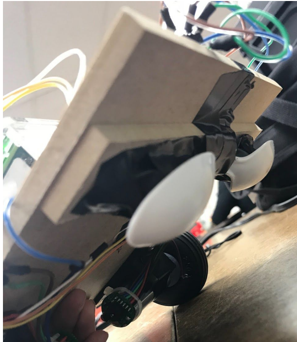
Figure E3: Plastic spoons added as skids, replacing the back wheels.
