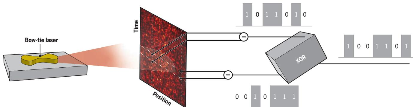
Kim *et al.* introduce another approach based on adapting the shape of the cavity. After performing extensive numerical modeling, the authors chose a bow-tie shape and precisely microfabricated a laser chip. The authors managed to boost the number of modes, avoiding their locking, and thereby substantially reduced the spatial and temporal correlation scales to 1.5  $\mu\text{m}$  and 2.8 ps, respectively.
