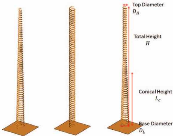
Figure 2 - From left to right: conical helical antenna, uniform diameter helical antenna and non-uniform helical antenna
