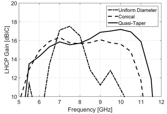
Figure 3 - Simulated boresight LHCP gain of the uniform diameter helical antenna, conical helical antenna and the quasi-taper antenna system.
