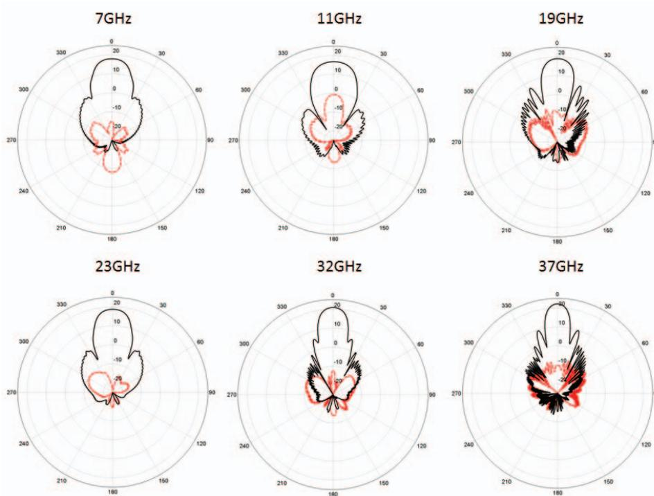
Figure 11 - Simulated pattern @ 7GHz, 11GHz, 19GHz, 23GHz, 32GHz and 37GHz. The Black Solid Line is the LCHP; The Red Dash Line is the RCHP
