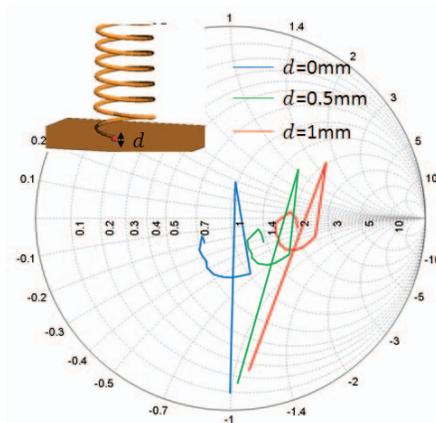
Figure 8 - Simulated helix impedance for different vertical feed heights.
