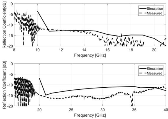
Figure 10 - Simulated and measured reflection coefficient data of mid-band and high-band antennas.
