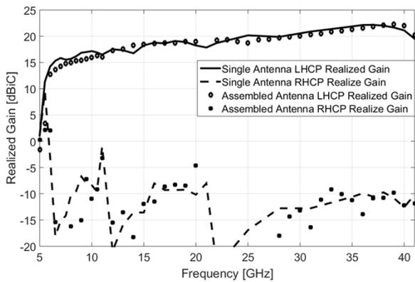
Figure 6- Simulated boresight realized gain of the single antenna and the assembled antenna system.
