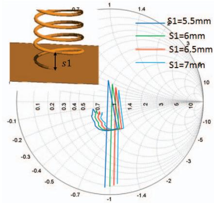
Figure 7 - Simulated helix impedance for different pitches in the first turn.
