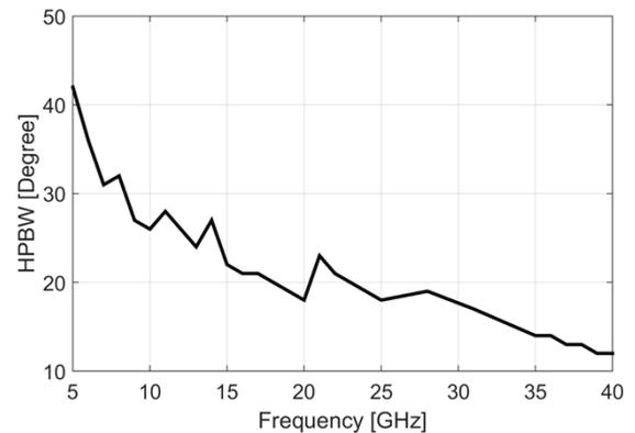
Figure 4- Simulated HPBW versus frequency.
