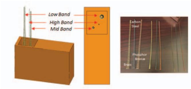
Figure 5 – (Left) CubeRRT antenna system on 6U CubeSat (Right) Fabricated quasi-tapered helical antenna elements made of different conducting materials: copper, brass, and steel.
