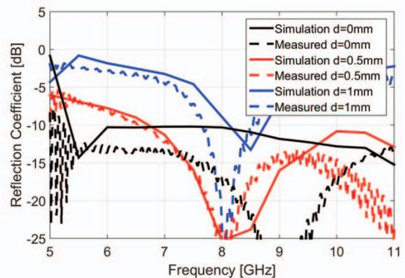
Figure 9 – Simulated and measured reflection coefficient data of low-band antenna for different feed heights.
