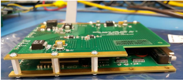
Figure 3. RDB engineering test unit (5" wide, 3.9" deep) with power board above and FPGA board below
