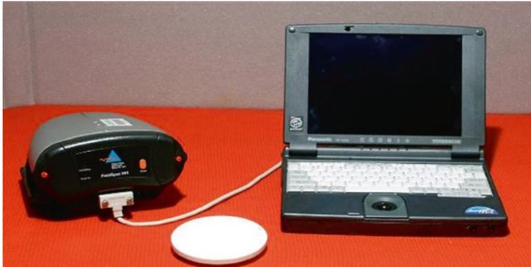
**Fig. 13.2** A FieldSpec HandHeld portable spectroradiometer (Analytical Spectral Devices, Denver) (*left*), a reference panel (*middle*), and a laptop computer
