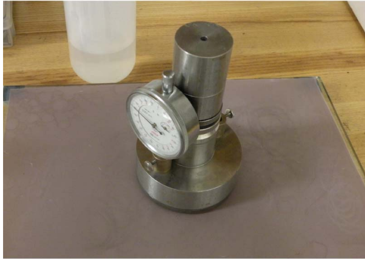
FIG D.1 Sample polishing with the pad.
