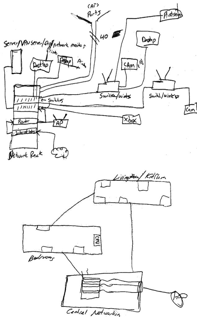
**Figure 1: Two sketches of the same network. The guru (top) depicts individual technical components of the network infrastructure, whereas the consumer (bottom) describes the backbone of the network as a single entity called “central networking”.**
