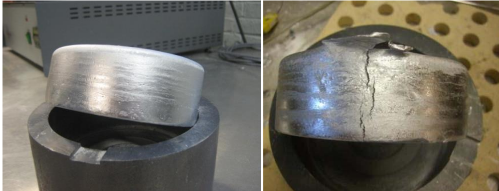
Fig. 7. (a) 2014 Cast via CDS - Free of Hot tears. (b) 2014 conventionally cast - Moderate hot tear.
