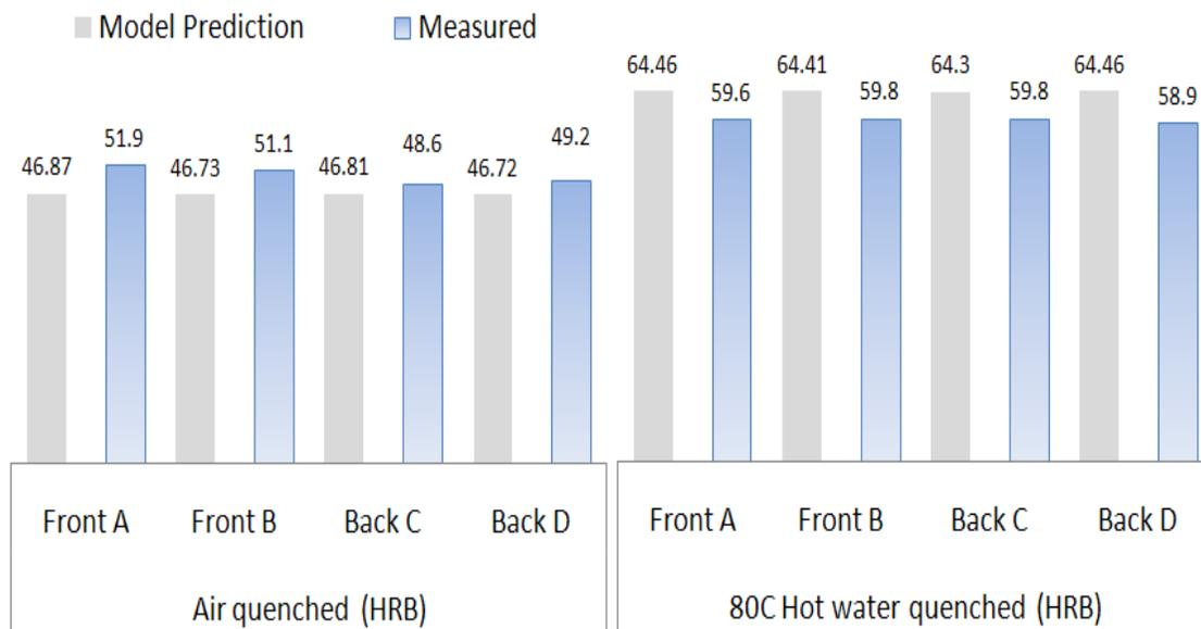
**Fig. 3** Measured and computer-predicted hardness for water quenched and air quenched cast parts.
