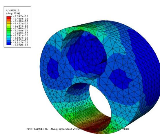
**Fig. 5** Computer-predicted properties of specimens quenched in forced air.
