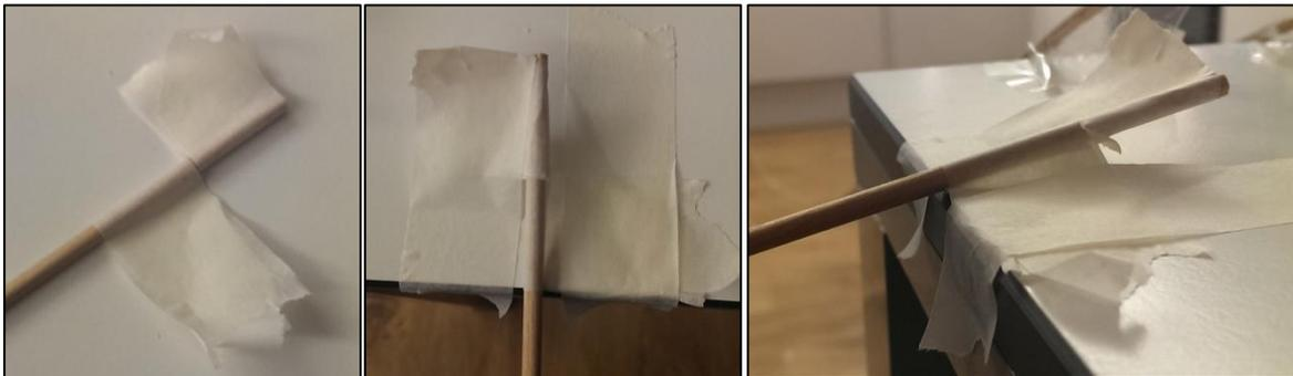
**Figures C, D and E:** This is one way to tape the rail to the desk at an angle. It uses 4 pieces of tape. Two are applied directly to the rod; they are then taped to the desk.
