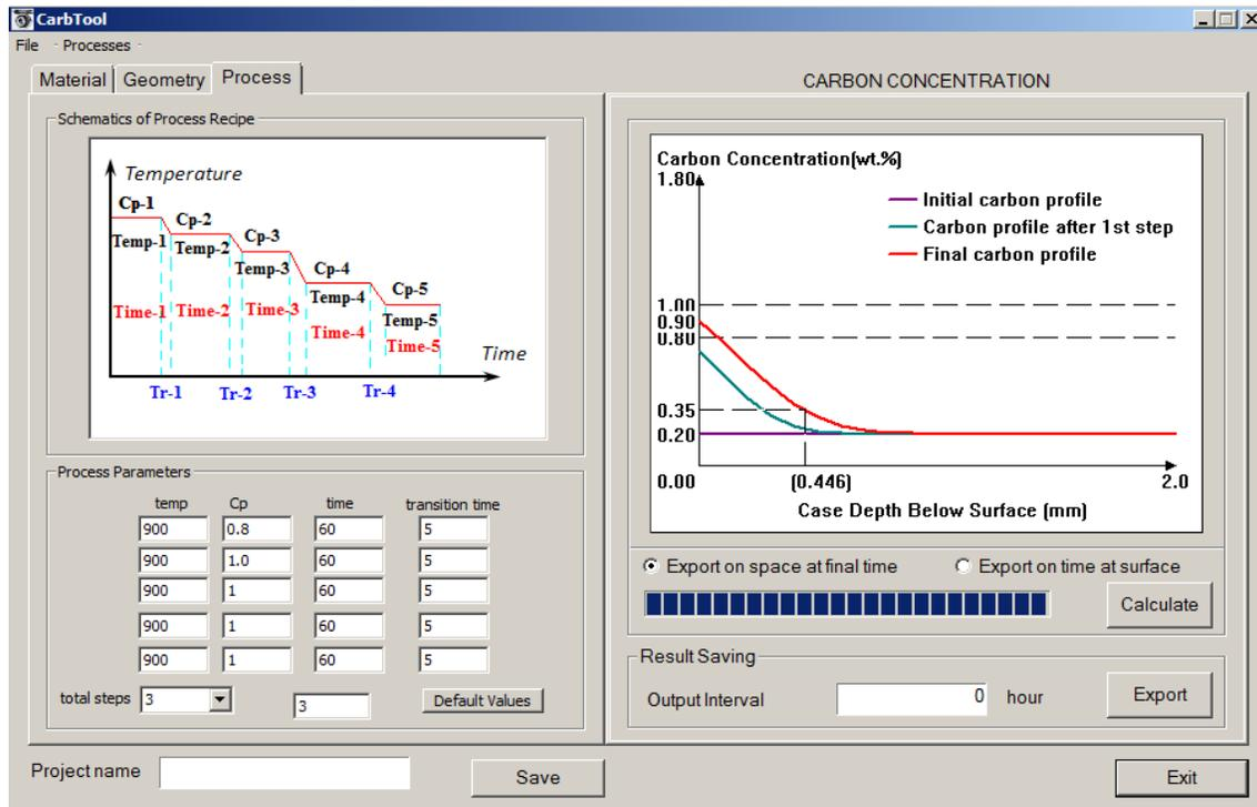
Figure 2 The interface of CarbTool, gas carburizing process module
