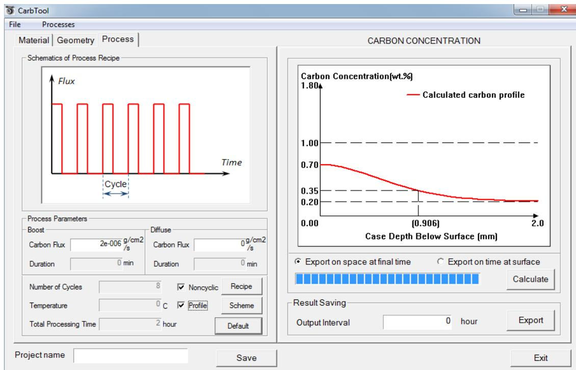
Figure 1 The interface of CarbTool, vacuum carburizing process module
