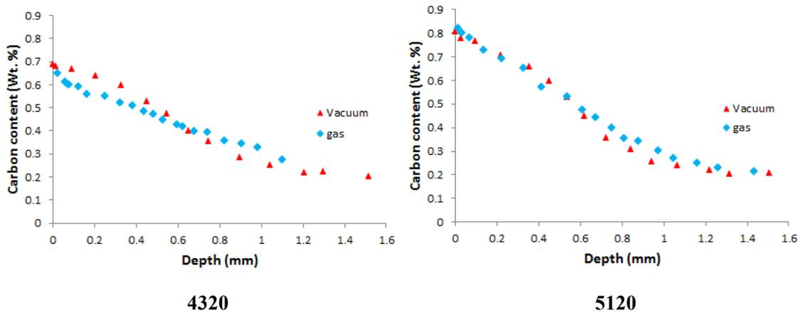
Figure 3 comparison between gas and carburized samples.
