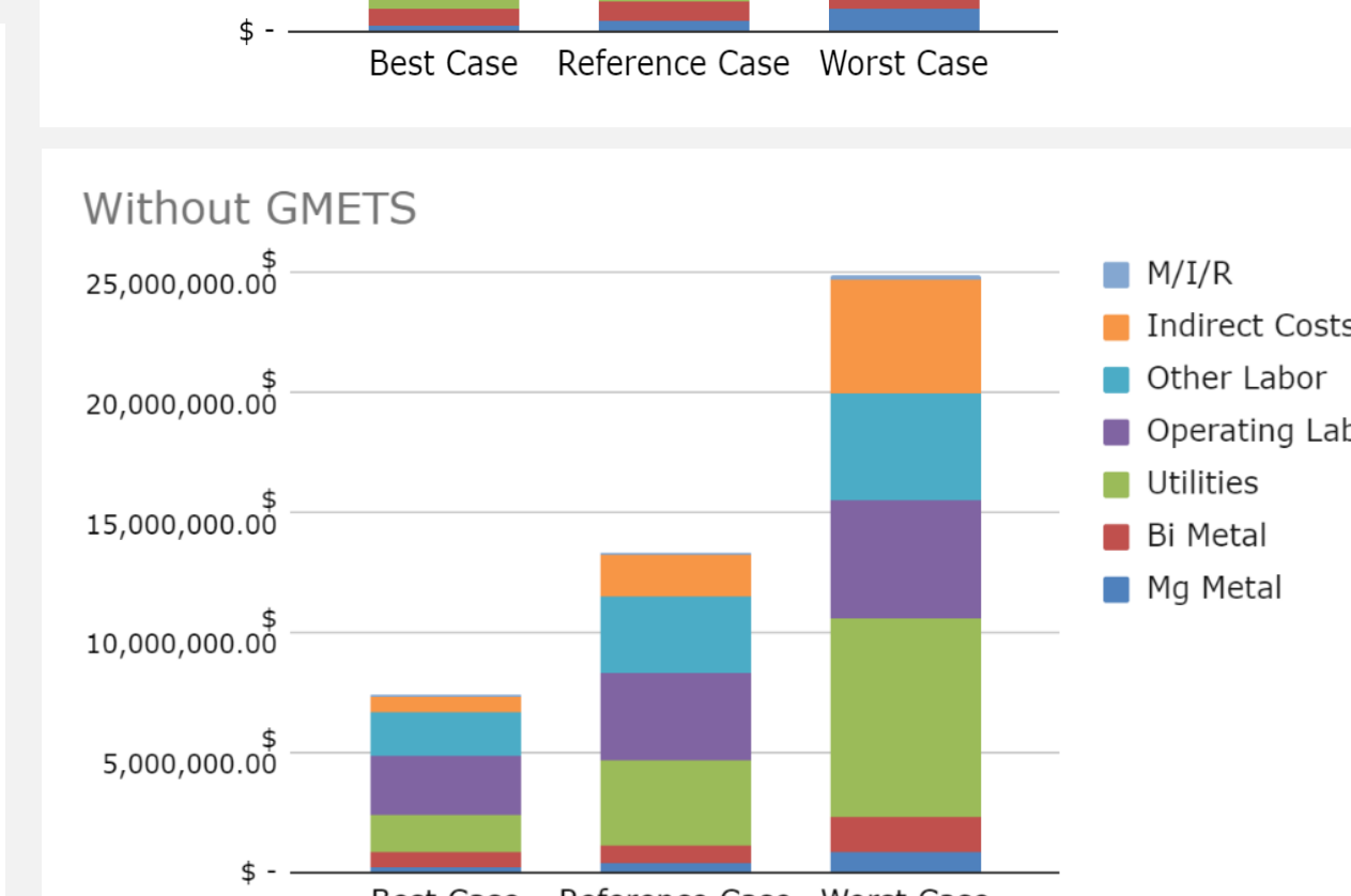
Figure 5: Three annual operating cost stack scenarios for a 205 t/year RE alloy recovery and further 11 t/year of Dy (using bismuth) with and without GMETS as well as conventional distillation. *M/I/R, maintenance/insurance/royalties.
