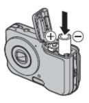
Slide tab over and swing up. Insert batteries correct end up as indicated. Put remaining batteries on the charger!
